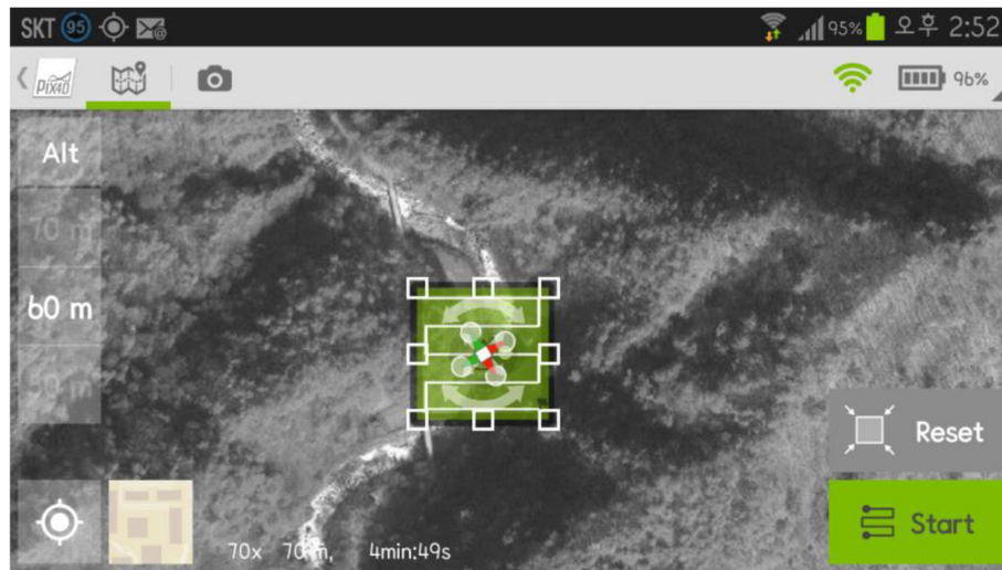
Fig. 3 Automatic flight mission grid of the UAV. The UAV follows the grid lines automatically set by Pix4D capture mapper application
