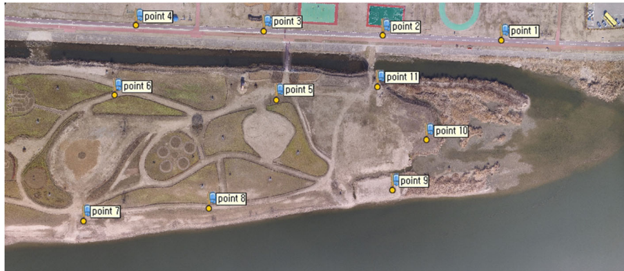
Fig. 2 Locations of ground control points (GCPs) installed in the study area
