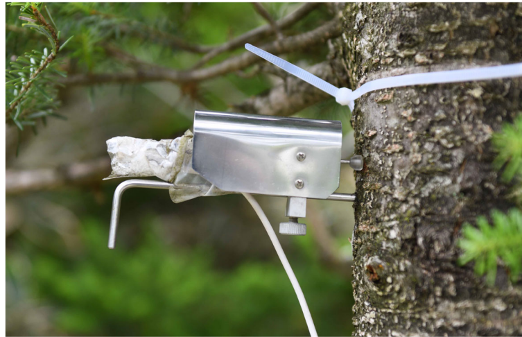
Fig. 2 Photo of the dendrometer installed on the stem of a Korean fir tree at the study site
